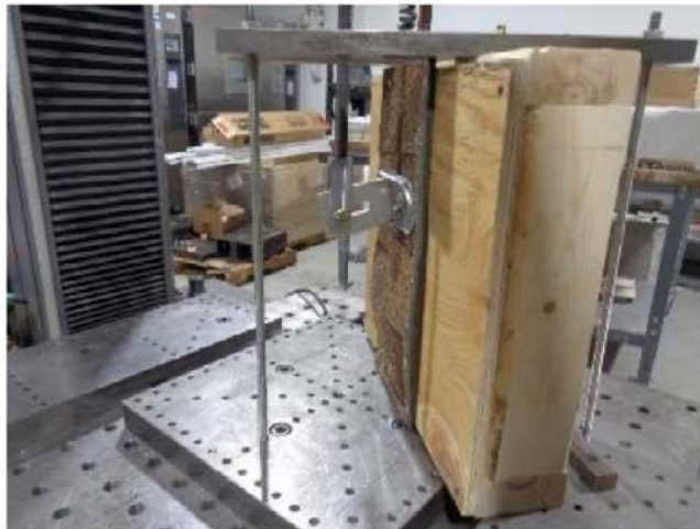
Photo No. 8 ASTM D7147 - Configuration F2 Test in Progress
