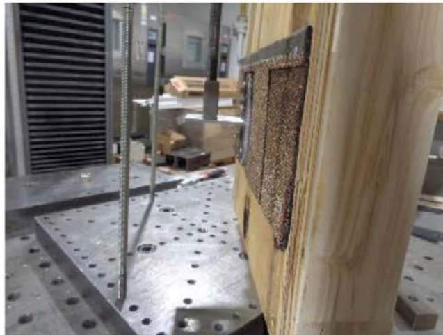
Photo No. 4 ASTM D7147 - Configuration F3 Test in Progress
