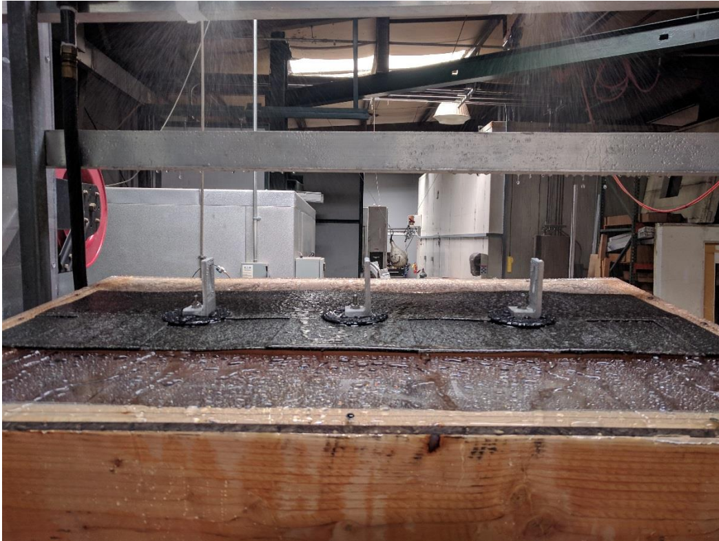
Photo No. 2 The specimen during ASTM E331 testing.
