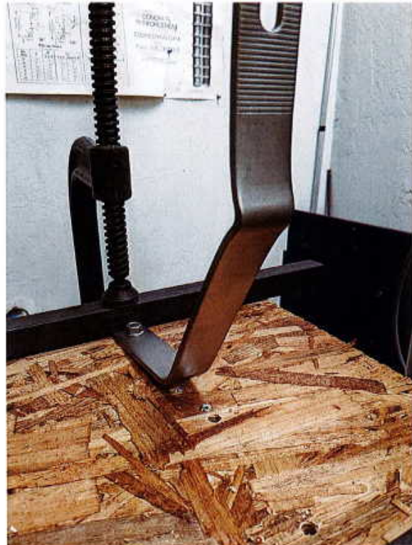
Figure 3b. Typical failure mode.
