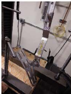
Photo 3: Typical Failure Mode - Fastener Pullout
