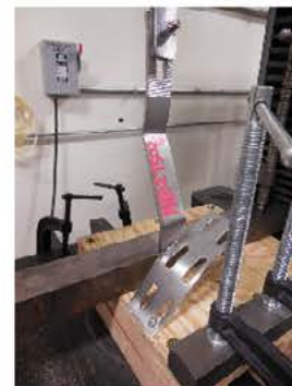
Photo 4: Typical Failure Mode - Fastener Pullout
