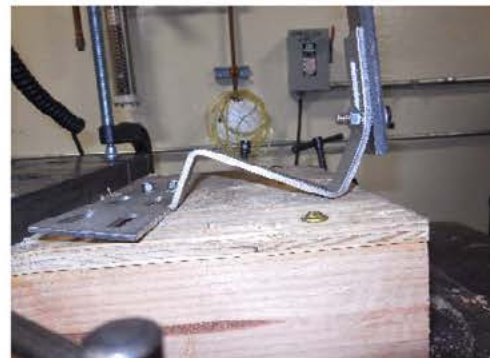
Photo 8: Typical Failure - Contact with Plywood
