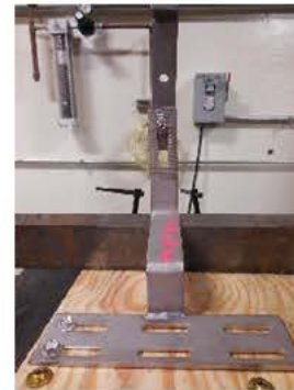
Photo 2: Tensile Test Setup
