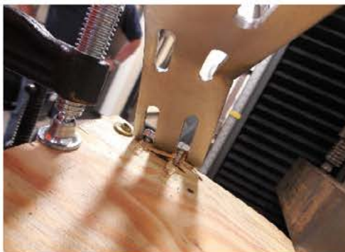
Photo 3: Closeup of Fastener Pullout
