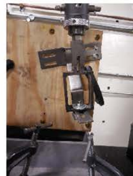
Photo 12: Typical Failure Mode - Deformation at Weld
