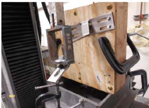
Photo 11: Deformation of Hook at Weld
