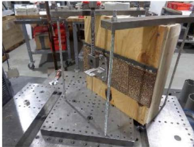
Photo No. 3 ASTM D7147 - Configuration F3 Test Setup
