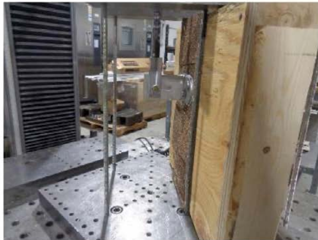
Photo No. 6 ASTM D7147 - Configuration F2 Test Setup
